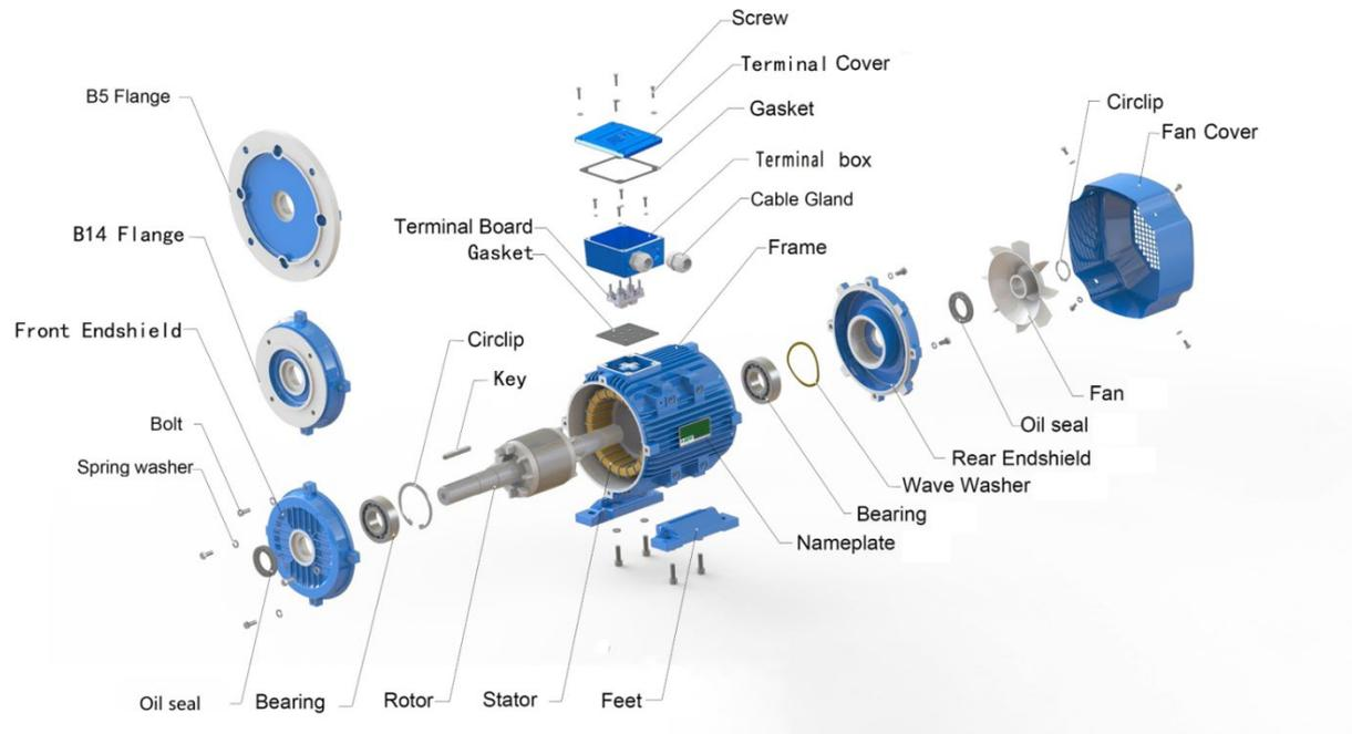
Picture 1. Typical exploded view of motors with sealed bearings.
