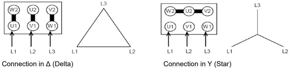
Figure 24. Standard three phase single speed motor.
