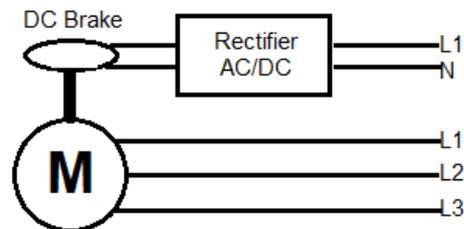
Figure 10. Example of DC brake motor connection
