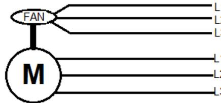
Figure 9. Example of three phase forced cooling connection.
