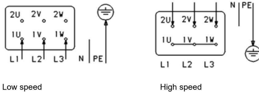
Figure 25. Three phase dual speed motor with single winding (Dahlander), like 4/2-, 8/4-, 12/6-pole.
