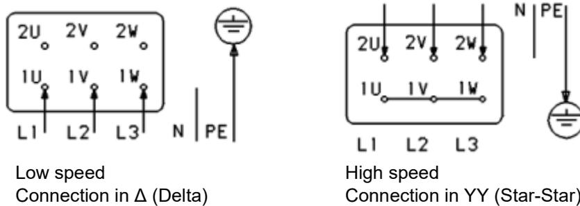
Figure 4. Three phase dual speed motor with single winding (Dahlander), like 4/2-, 8/4-, 12/6-pole.
