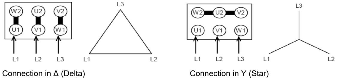
Figure 20. Standard three phase single speed motor.
