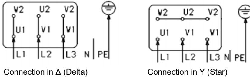
Figure 11. Standard three phase single speed motor
