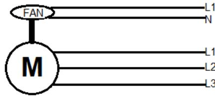
Figure 8. Example of single phase forced cooling connection.
