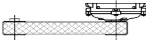
Figure 3 Illustration of belt mounted on shaft
