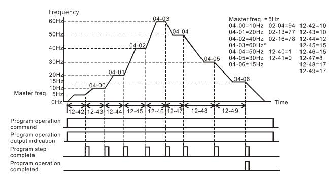
The diagram above shows one complete PLC cycle. To restart the cycle, turn the PLC program off and then turn back on.
