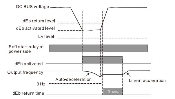
Situation 3: Power supply unexpected shut down or power loss.
