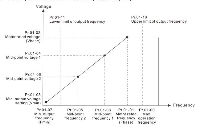
The lower output frequency limits the minimum output frequency of the drive. When the drive frequency command is lower than this setting, the lower limit of the frequency limits the drive output frequency.
