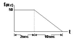
Therefore, the distance travelled by the motor after the STOP command is given = number of revolutions x circumference =  $175x 2 \pi$  r. It means the turntable returns to the top after 175 revolutions.
