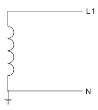
4. No stable neutral grounding in a three-phase autotransformer configuration
