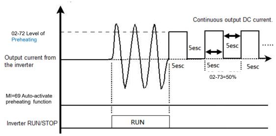
The figure below shows the timing relationship between preheating function and enabling DC brake.
