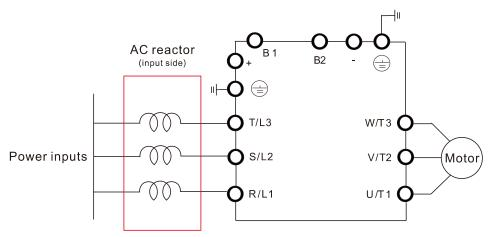
Connecting an AC input reactor
