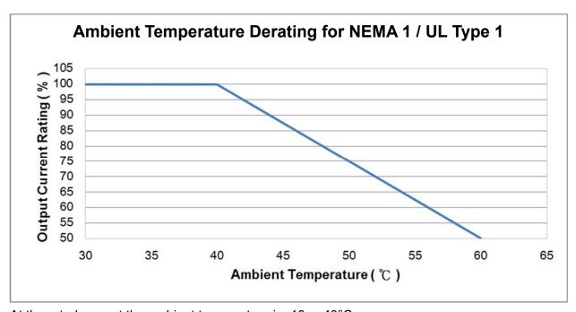
At the rated current the ambient temperature is -10- +40°C.
