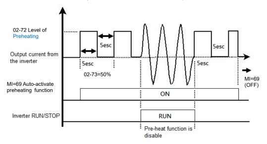
The figure below shows the timing relationship when MI=69 auto-activate preheating function is disabled and when preheating DC current is enabled and cycle time is 50%. When the motor drive is stopped, the preheating function starts to output DC current continuously.
