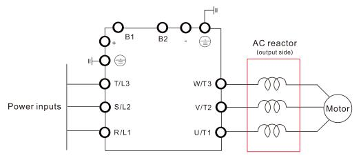
Connecting an AC output reactor
