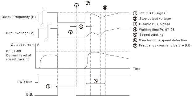
B.B. Speed tracking: from last output frequency
