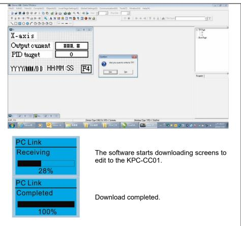
2. VFDSoft: this function links to the VFDSoft Operating software, and then you can upload data.
