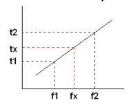
$$\mathbf{t}_{x} = t_{1} + \left(\frac{f_{x} - f_{1}}{f_{2} - f_{1}}\right) \times (t_{2} - t_{1}) = t_{1} + \left(\frac{f_{x} - f_{1}}{10}\right) \times (t_{2} - t_{1})$$
