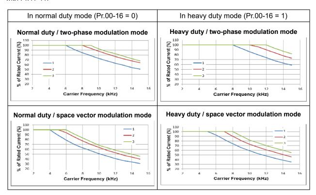
**NOTE** Line 1:  $T_a = 50^{\circ} \text{ C} / \text{ Duty} = 100\%$
