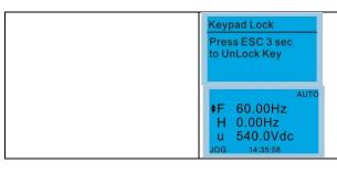
At this time, press any key on the keypad, and a message displays as shown on the left.
