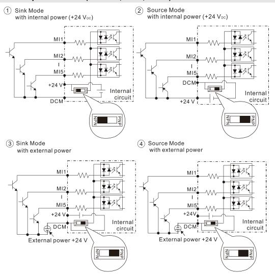
☑ When the photo coupler is using the internal power supply, the switch connection for Sink and Source modes are as shown in the picture above: MI-DCM: Sink mode, MI+24 V: Source mode.
