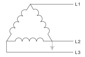
2. Grounding at a midpoint in a polygonal configuration
