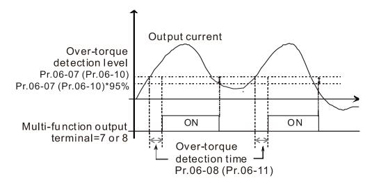
When you set Pr.06-06 or Pr.06-09 to 2 or 4, an ot1 / ot2 warning displays and the drive stops running after over-torque detection. The drive keeps running after you manually reset it.
