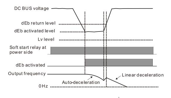
Situation 2: Momentary power loss, or power current too low and unstable, or power supply sliding down because of sudden heavy load.
