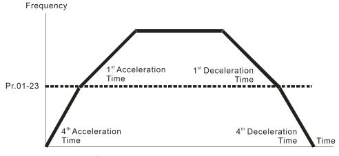
1<sup>st</sup>/4<sup>th</sup>Acceleration/Deceleration Frequency Switching
