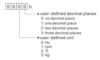
You must convert the setting value to decimal when using the keypad to set parameters.
