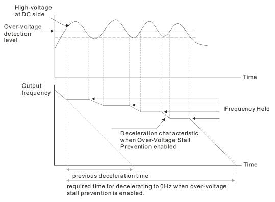
When you set Pr.06-02 to 1, to use smart over-voltage stall prevention during deceleration, the drive maintains the DC BUS voltage when decelerating and prevents the drive from OV.
