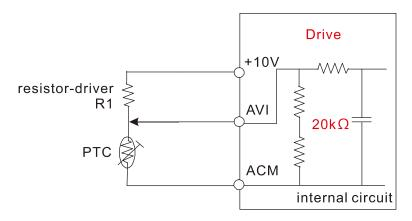
Take the standard PTC thermistor as example: if protection level is  $1330\Omega$ , the voltage between +10V-ACM is 10.5V and resistor-divider R1 is  $4.4k\Omega$ .
