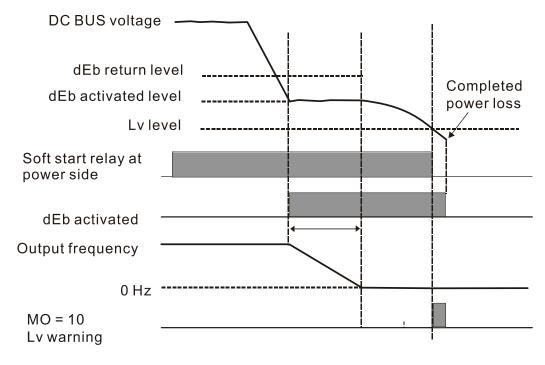
Situation 4: Power supply unexpected shut down or power loss.
