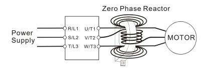
Figure B: Multi-turn zero phase reactor
