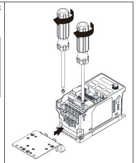
2. After selecting a suitable R-clip according to the wire gauge used, fix the R-clip on the shield plate.
