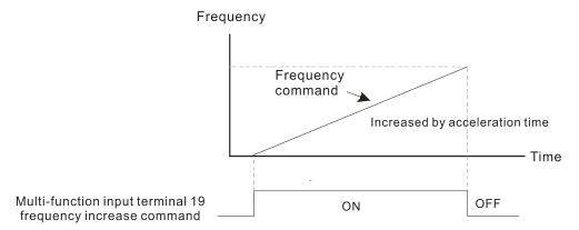
When Pr.02-09 is set to 1: the increasing / decreasing frequency command (F) operates according to the setting of Pr.02-10 (0.001–1.000 Hz/ms).
