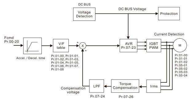
When Pr.00-10 = 0 and you set Pr.00-11 to 2, the sensorless vector control diagram is as follows:
