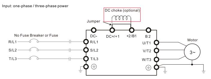
Wiring of DC reactor
