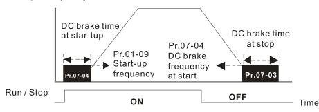
DC Brake Output Timing Diagram
