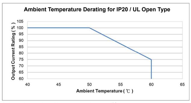
At the rated current the ambient temperature is -10- +50°C.
