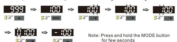
The upper limit for Pr.03-03 is 100.0 and lower limit is -100.0. If the value is more than 100.0 or less than -100.0, "Err" appears after you press the digital dial, and then the keypad shows the upper limit (100.0) or lower limit (-100.0) for a second to remind you of the incorrect setting. The setting value remains as the original set value, and the cursor returns to the last digit.
