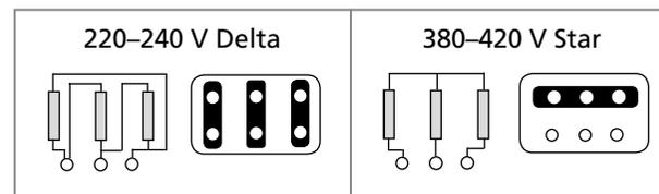
a) 220-240 V Delta/380-420 V Star - may be labelled 230/400 V (standard for motors 3 kW and smaller). Suitable for direct on line starting on 380-420 V supplies.
