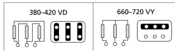
b) 380-420 V Delta/660-720 V Star - may be labelled 400 V Delta (standard for motors 4 kW and larger). Suitable for Star/Delta starting on 380-420 V supplies or direct on line starting on 660-720 V supplies.
